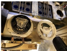
New design of marking loading plates for laser marking station MQB2020 (90mm with 100mm)
